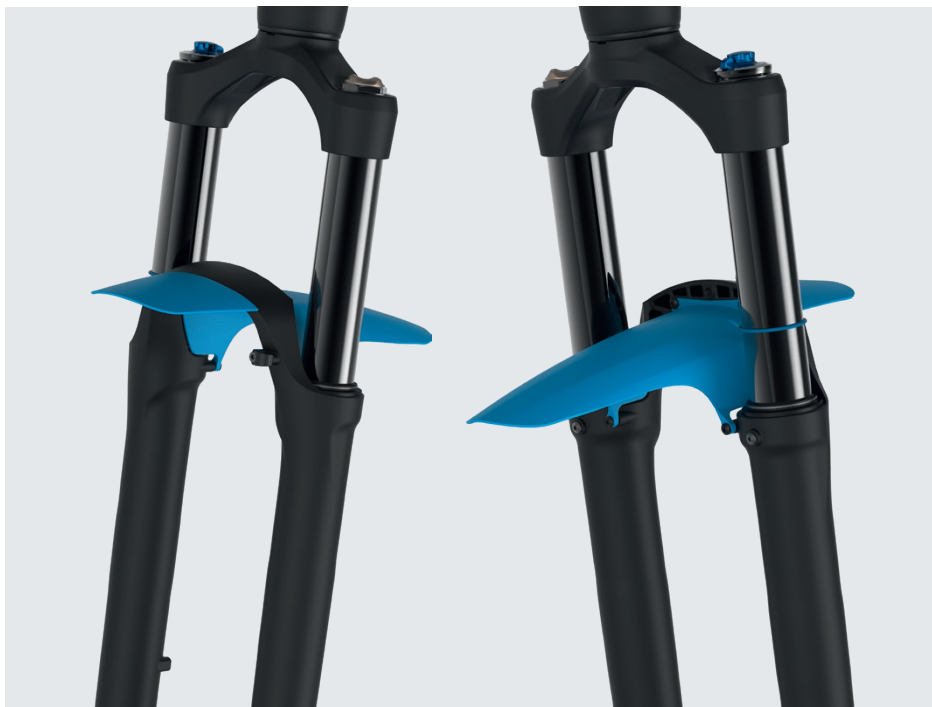
SHORT FENDER MOUNT Detachable integrated short fender
