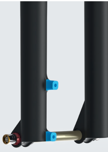
DS POSTMOUNT DISC BRAKE TYPE
