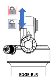
The operation of remote lockout function can be done from the remote lever on the handlebar, while gripping the grip without taking your hand off from the handlebar. The remote lever is to use the lock and unlock function.
