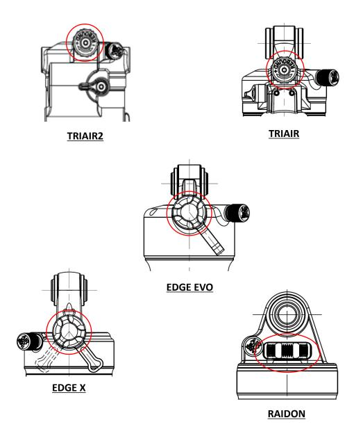
Rebound controls the speed at which the shock extends after compression. Rebound damping control is relative to the main spring rate. Higher pressures require more rebound damping. Lower pressures require less rebound damping, so please adjust accordingly.
