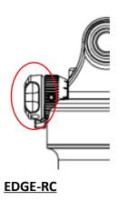
The compression damping adjust function of your SR SUNTOUR rear shocks allows you to tune your shock according to your personal preferences and the terrain you are riding on. This function controls the speed of your rear shock while being compressed.
