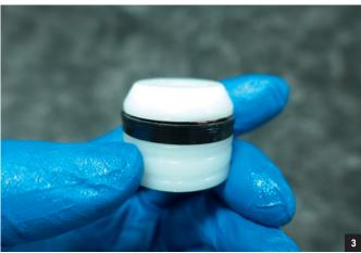
Apply some SR SUNTOUR "Low-Friction" grease to the inside of the stanchion and on the piston seal. Grease the coil springs with SR SUNTOUR "Low-Friction grease". Install both the screw and the piston on the negative shaft assembly.
