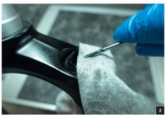
Compress the air shaft all the way to make sure no air is left in the chamber. If you feel resistance, apply pressure on the shaft and release the air from the top valve.
