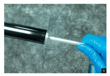
Grease the inner surface of both dust seals and bushings with SR SUNTOUR "Low-Friction" grease.
