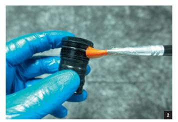
Inject 3cc of Air chamber oil directly in the stanchion.
