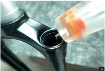
Install the air cap assembly in the left stanchion. Use the dedicated 27mm socket and ratchet and tighten to 15Nm.
