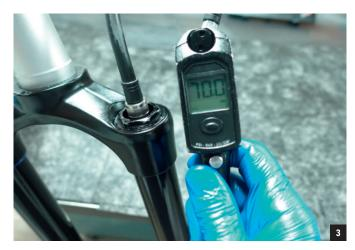
Manipulate the air shaft to make sure it is centered. You might hear a "clack" noise; this is normal as it helps the shaft head to align with the air piston.
