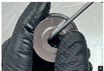
Make sure the seal is seated correctly without any twists.
