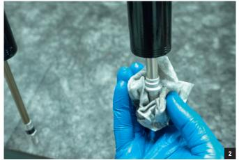
Slide the spacer, bumper, and nose piece down to expose the shaft. Clean the shaft with brake cleaner and a workshop towel. Use 10 mm clamps to hold the shaft in a vise.
