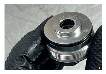
Remove the O-ring and set it aside. Clean the seal seat, apply grease to the new O-ring, then install it.
