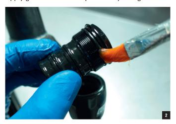
Install the air cap assembly in the left stanchion using the dedicated 27 mm socket and ratchet, and tighten to 15Nm.
