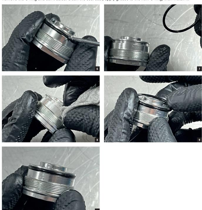
Hold the piston and remove the two backup rings and the x-ring seal. Clean the piston.
