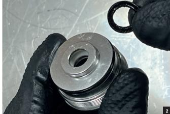
Clean the seal seat with a rag. Grease and install the new x-ring.
