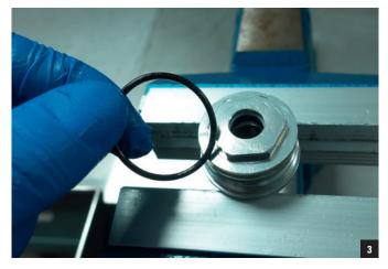
Use a 21mm socket or wrench to loosen the top nut by turning it counterclockwise. Remove the top nut and its inner o-ring seal. Remove the white backup rings and the x-ring seal.
