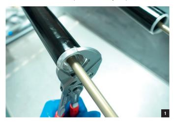
Move the nose piece partway down the shaft (picture 1). Pull the shaft and remove the air shaft assembly. Set it aside (picture 2).
