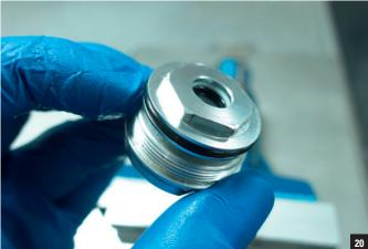
Use a torque wrench with a 21mm socket and tighten to 6Nm.
