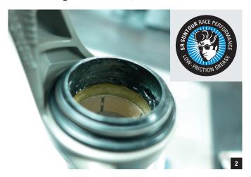
Install the lower legs. Refer to the procedure "LOWER LEGS SERVICE..." specific to your fork. In summary, make sure the o-rings are installed at the bottom of both the air shaft and damper shaft respectively. Pull the damper shaft to the bottom of the stanchion, then install the lower legs onto the stanchions.
