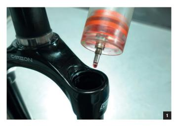
Apply grease to the air cap assembly o-ring.
