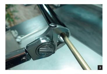
Inject 1-2cc of air chamber oil directly in the stanchion.
