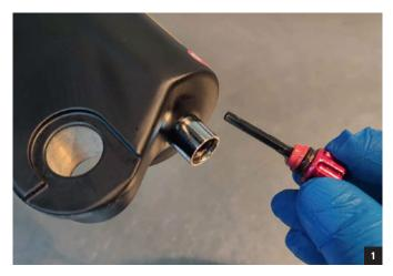
Using an 8mm Allen key, turn the exposed bolt counterclockwise 2 turns to loosen it.
