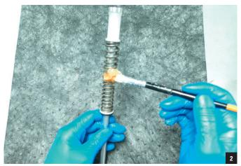
Clean the air cylinder, then apply a thin coat of SR SUNTOUR "Low-Friction" grease to the cylinder. Install the negative spring assembly and the piston.
