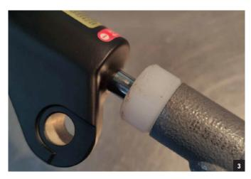
On the air/spring side, using a 5mm Allen key, turn the bolt counterclockwise 3-4 turns to loosen. Use a mallet to strike the bolt 2-3 times. Check to ensure the bolt is in contact with the leg. Remove the bolt and set it aside. Pull on the lower legs to remove them, and set them aside.
