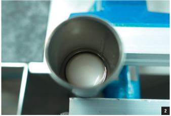
Install the air cap assembly on the air cylinder and slide the assembly into the left stanchion. Use the dedicated 27mm socket and ratchet to tighten to 15Nm.
