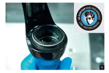
Clean the stanchions. Fully extend the damper cartridge and install the lower legs.
