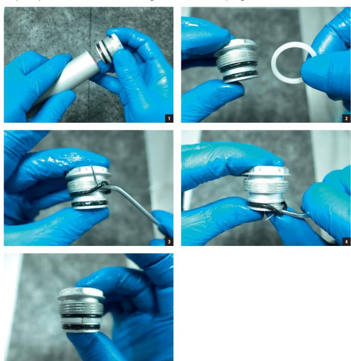
Push in the negative spring shaft and remove the air piston and negative spring assembly.
