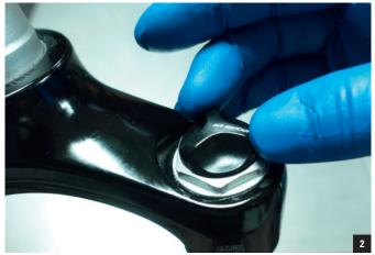
Manipulate the air shaft to make sure it is centered. You may hear a "clack" sound; this is a normal result of the shaft head aligning with the air piston.
