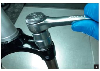
Pressurize the air chamber and re-install the air cap.
