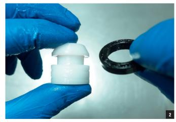
Clean the piston. Grease the new seal and install it by hand onto the piston. Make sure to install the seal in the correct orientation.
