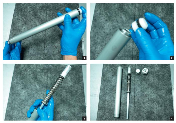
Remove the piston seal.
