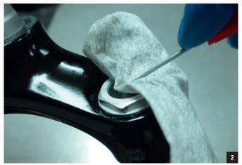
Use the dedicated 27mm socket and a ratchet to unscrew the Air cartridge from the crown. Carefully remove the air cartridge from the stanchion and set it aside.
