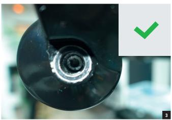
First thread the bolt in by hand then use an 8mm Allen key to tighten the bolt to 12Nm.
