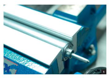
Position the threaded plastic adjuster, the washer and the steel bolt.
