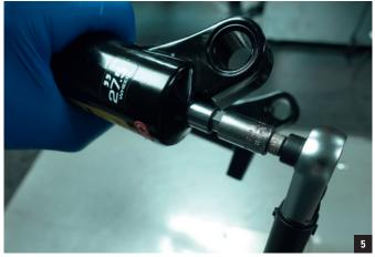
Use a 3mm Allen key to set the rebound to fully-open (turning it counterclockwise) then close it by 1-2 turns (turning it clockwise). Remove the Allen key and reinstall the rebound adjuster knob by pressing it into the bolt.
