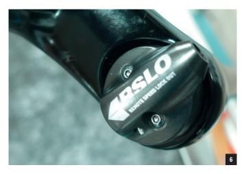
6. RL-R cartridge: Make sure the damper cartridge shaft is aligned with the lower leg hole. If not, use a 3mm Allen key to center the shaft.
