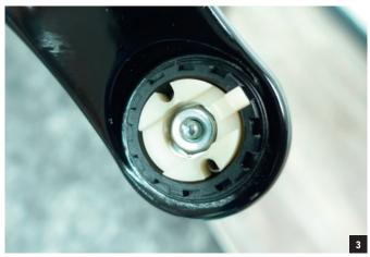
Grease the steel sliding component. Install the RSLO cover assembly and use a 2mm Allen key to tighten
