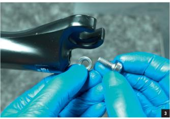
RL-R cartridges: On the damper side, pull on the rebound adjuster knob to remove it, then set it aside. Using an 8mm Allen key, turn the exposed bolt counterclockwise 2 turns to loosen it.
