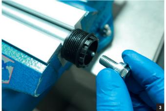
Use a torque wrench and tighten to 10Nm.
