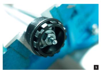
**5**. Install the cartridge in the crown and tighten with the FAA122 tool. Install the plastic guide.
