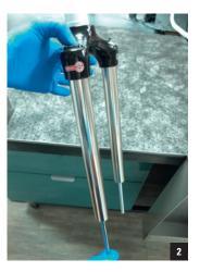
Press and hold the pin, maintaining pressure. With the pin pressed, try to compress the fork (or damper shaft if the lower legs have been removed). It should not compress. If it does move, compress the fork/ cartridge 8-10 more times. Release the pin, press it again, then attempt to compress the fork/cartridge shaft again. If the fork/cartridge still compress, it must be replaced. Go to point "2".
