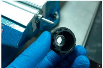
4. Remove the cartridge from the Vise. Position the new cartridge in the aluminium jaws as shown on the image below.
