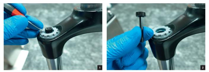
**3.** On the damper side, using a 5mm Allen key, turn the lower-leg bolt counter clockwise 2 turns to loosen it. For HLO and NLO version, use a 10mm socket to remove the nut following the same process.
