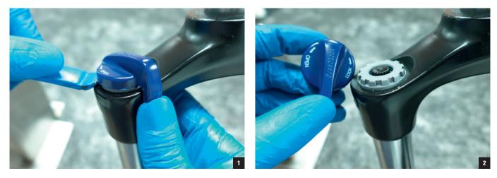
**2**. Use a small flat (slotted) screwdriver to remove the adjust core and set it aside.
