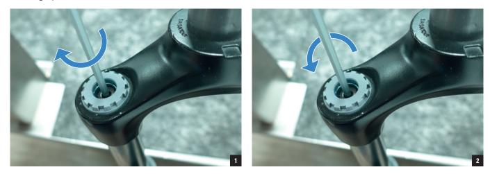
**4.** Insert the 4mm Allen key again and gently turn clockwise to set the cartridge into the "Locked" position (picture 1). Remove the Allen key and check the lockout function of the fork as described in point "**3**".
