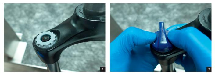
6. Turn the lockout knob 180° counter clockwise to unlock the fork.
