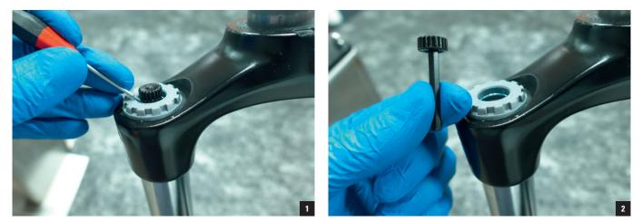
**3.** Check the cartridge position: insert a 4mm Allen key through the black bolt and gently turn clockwise until it stops (picture 1). Do not use force. The cartridge is now in the "Locked" position. Now turn the Allen key  $\frac{1}{2}$  turn (180°) counter clockwise to set the cartridge to the "Open" position (picture 2).
