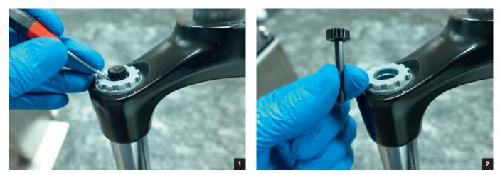
**3**. Insert a 4mm Allen key through the black bolt and gently turn clockwise until it stops (picture 1). Do not use force. The cartridge is now in the "Lock" position.
