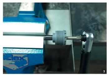
**7.** Remove the cartridge from the vise. Use a 4mm Allen key to set the cartridge in the open position (refer to point "**1-3**").
