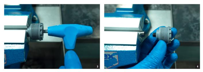
**6**. Remove the cartridge from the vise and install the new one as shown in the images below. Install the adjust system and tighten to **7Nm**.
