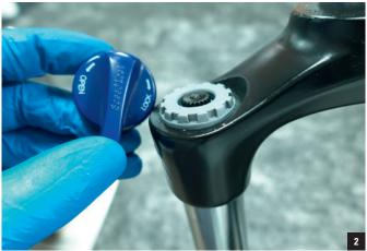
**2**. Use a small flat (slotted) screwdriver to remove the Adjust core and set it aside.
