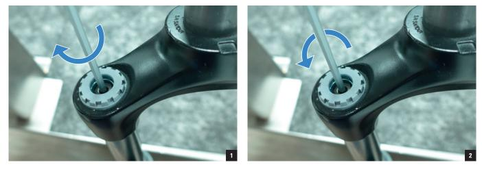
4. Remove the Allen key and check the lockout function of the fork.
