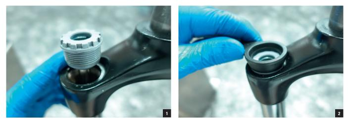
8. Install the washer and bottom bolt and tighten to 8Nm.
