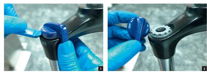
2. Use a small flat (slotted) screwdriver to remove the adjuster core and set it aside.
