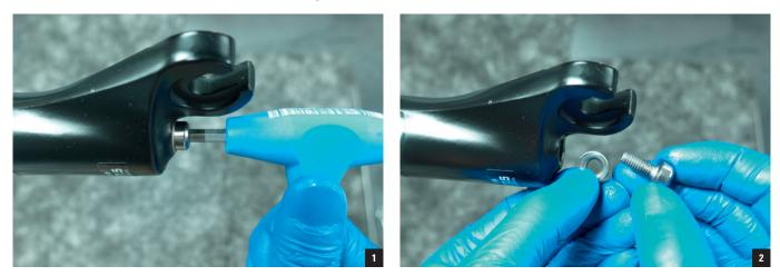
**9.** Insert a 4mm Allen key through the black bolt and gently turn clockwise until it stops (picture 1). Do not use force. The cartridge is now in the "Lock" position. Install the adjuster core.
