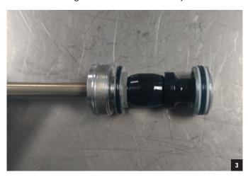
Apply SR SUNTOUR "Low-Friction" grease to the piston x-ring seal, the nose piece O-ring, and the inside of the stanchion.
