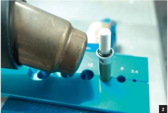
Use a 2.5mm steel shaft or 2.5mm Allen key to loosen the threaded insert by turning it counterclockwise.
