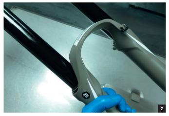
Pressurize the air spring to 70 psi and equalize the positive and negative chambers by compressing the fork a few times within the sag portion of the fork travel.
