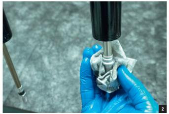
Slide the spacer, bumper, and nose piece down to expose the shaft. Clean the shaft with brake cleaner and a workshop towel. Use 10mm clamps to hold the shaft in a vice.
