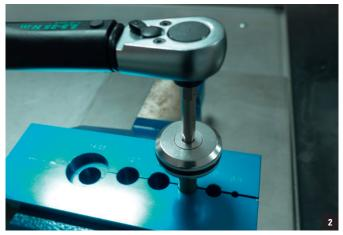
Remove the negative air shaft assembly from the clamps.
