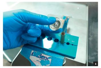
Remove the shaft from the vice. Remove the plastic spacer, rubber bumper and nose piece from the shaft and set them aside.
