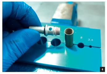
Clamp the new air shaft and install it in the vice. Make sure to install the shaft in the correct way (picture 3).
