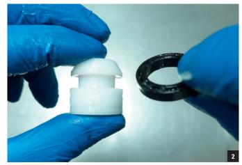
Clean the piston. Grease the new seal and install it by hand onto the piston. Make sure to install the seal in the correct orientation.
