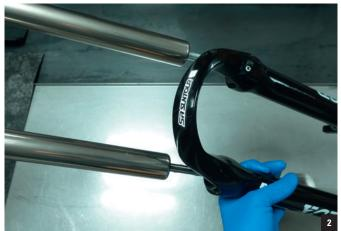
Make sure the damper cartridge shaft is aligned with the lower leg hole. If not, use a 3mm Allen key to center the shaft.
