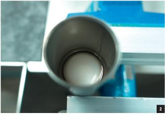
Install the air cap assembly on the air cylinder and slide the assembly into the left stanchion. Use the dedicated 27mm socket and ratchet to tighten to 15Nm.
