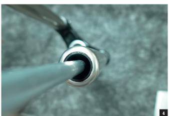
Replace or clean the dust seals. Clean and grease the bushings, and grease the dust seals using dedicated SR SUNTOUR "Low-Friction" Grease).
