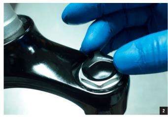
Manipulate the air shaft to make sure it is centered. You may hear a "clack" sound; this is a normal result of the shaft head aligning with the air piston.
