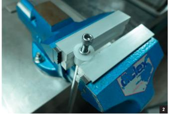
Use a mallet to strike the bolt. The shaft will slide down the spacer. Collect the shaft, remove the bolt and set it aside.
