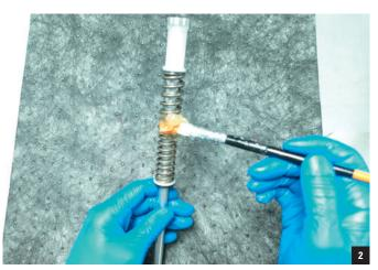
Clean the air cylinder, apply a thin coat of SR SUNTOUR "Low-Friction" Grease into the cylinder. Then install the negative spring assembly and the piston.
