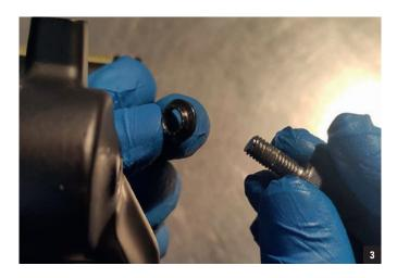
Remove the air cap and depressurize the air chamber by depressing the center pin of the Schrader valve.
