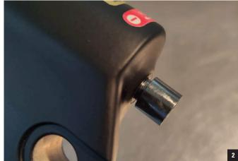
Use a mallet to strike the bolt 2-3 times. Check to ensure the bolt is in contact with the leg. Remove the bolt and set it aside.
