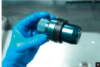
Hold the lower legs with one hand and finish the installation by tapping the installation tool with a plastic mallet. Once you hear a change in the tapping sound, remove the tool and check that the seal edge is flush with the lower leg. If necessary, repeat the process until the seal is flush with the lower leg. Install the new foam rings (picture 6).
