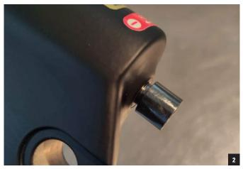
Use a mallet to strike the bolt 2-3 times. Check to ensure the bolt is in contact with the leg. Remove the bolt and set it aside.
