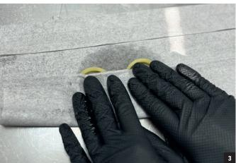
Soak the foam rings into 20wt oil for 5-10 minutes and reinstall them.
