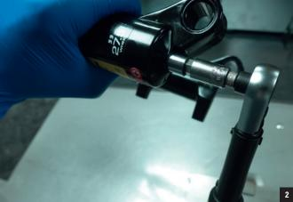
Use a 3mm Allen key to set the rebound to fully-open (turning it counterclockwise) then close it by 1-2 turns (turning it clockwise). Remove the Allen key and reinstall the rebound adjuster knob by pressing it into the bolt.
