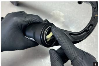
Grease the bushings and dust seals using the dedicated SR SUNTOUR "Low-Friction" grease.
