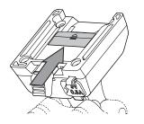
Slide up to cover the contacts and to prevent short circuits and malfunctions.
