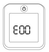
In the rare event of a system malfunction, an error message will appear on the display. If an error message appears, turn the system completely OFF and then ON. If the error message still appears, contact your local dealer for assistance.
