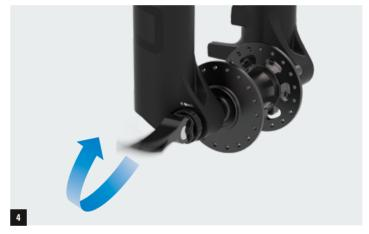
**4** Close the lever all the way. It should leave an impression in the palm of the hand. "Close" should face towards outside as shown in 4.
