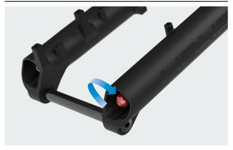
Rebound controls the speed of the fork extension after compression. Always start the rebound setting process with the rebound knob (located bottom of the drive-side of the fork) in closed position by turning the adjuster knob all the way to the end of the clock-wise position (+).
