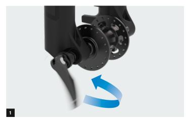
1 Open the lever. Turn the axle counter clockwise.
