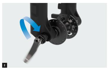
2 Turn the lever clockwise to tighten the axle until it stops. Do not turn with a torque greater than 10 Nm.
