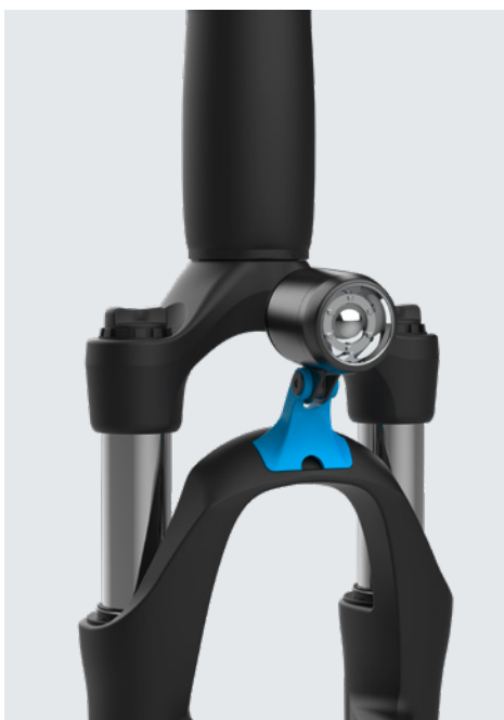
INTEGRATED TYPE ON FORK BRACE
