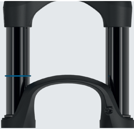
HARD ANODIZED BLACK A7 / A6000 series aluminum
